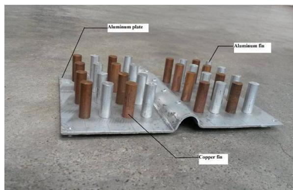
Fig 3.4 Aluminium plate with pin fins plate with
