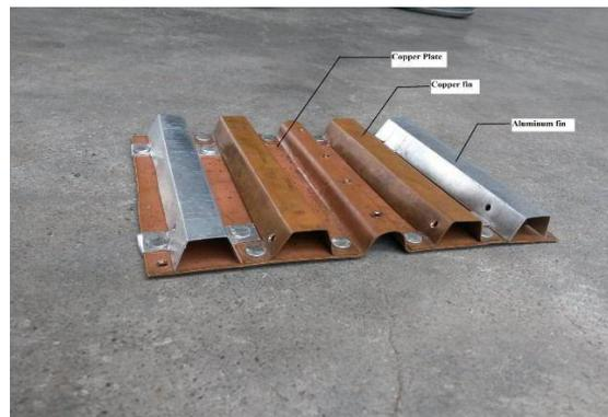
Fig 3.6 Aluminium plate with Trapezoidal fins
