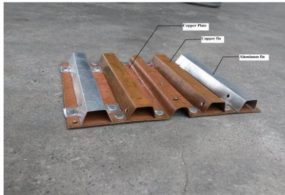
Fig 3.6 Aluminium plate with Trapezoidal fins
