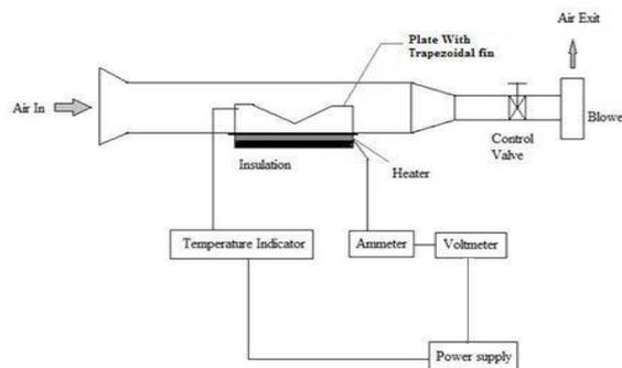
Fig. 3.1 Sketch of the experimental set up
