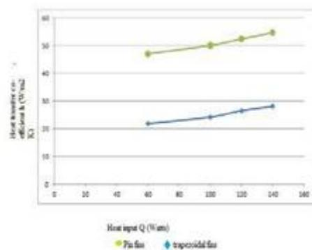
Comparison of Heat Transfer Co-efficient for aluminium plate with pin fins and aluminium plate with trapezoidal fins
