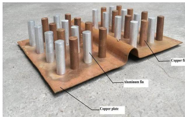
Fig 3.3 Copper plate with pin fins
